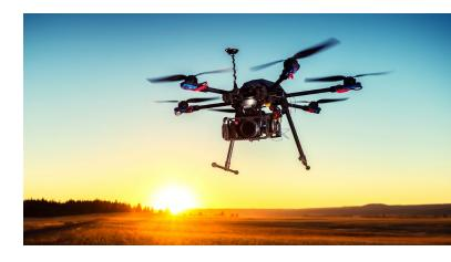
than 55 pounds (including equipment and cargo), stay below 400 feet in the air, and remain with the visual line of sight of a licensed operator.
